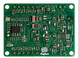
The LNBC series bias controllers provide salient performance enhancements. They enable the modulator's operation at the highest extinction ratio and independent of environmental changes. This is achieved by injecting a low-frequency, low-amplitude dither signal together with two built-in photodetectors to form a feedback bias control to maintain optimized performance and reduce temperature dependence. The bias is applied via an integrated micron heater.
